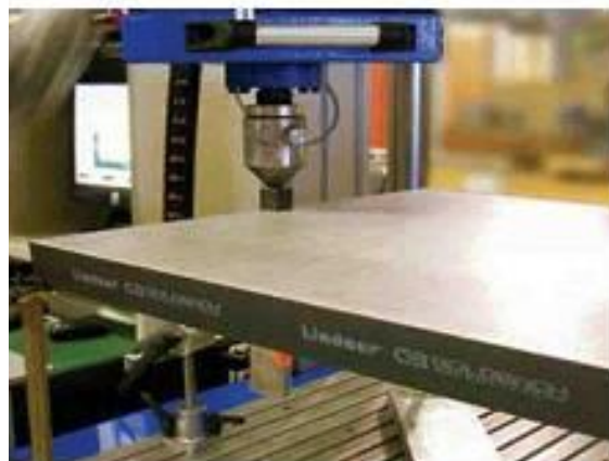
Inspection for load-bearing capacity.
